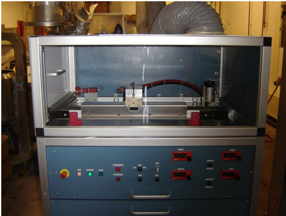
Figure 8: Plasma source and fibre processing systems placed in closed box with fume exhaust.
