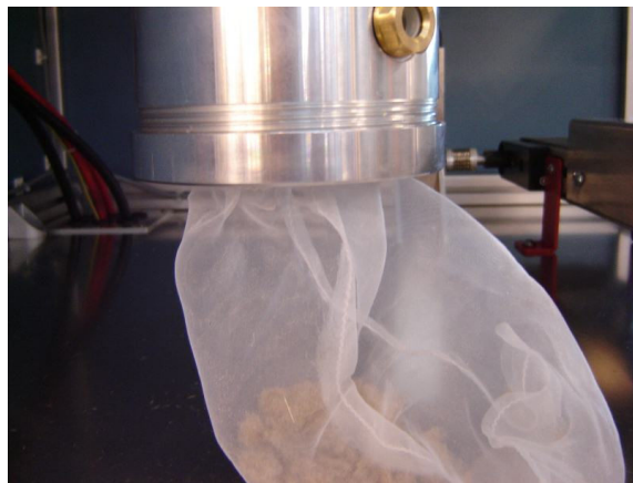
Figure 12: Gauze bag to collect fibres from the short fibre processing set up.
