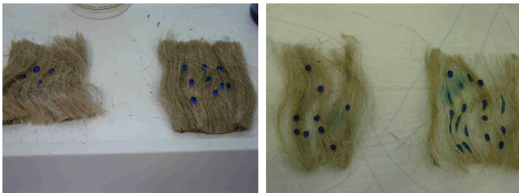
Figure 2: Water droplet absorption. Left fibre sample on each picture is the untreated reference, right fibre sample is the plasma treated fibre. Left picture does not show change of water absorption, the right picture does.
