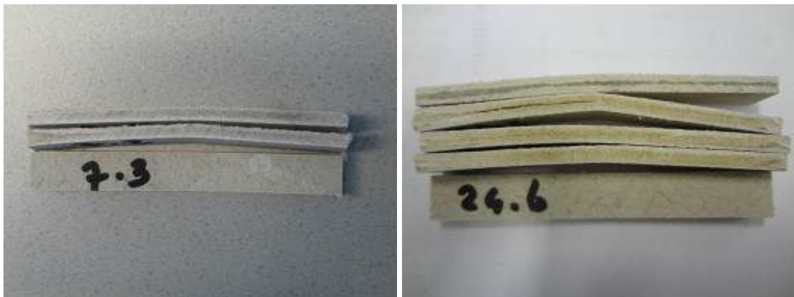
Figure 7: SMC specimens based on (steam exploded) flax fibre, the central section of the composite showing incomplete fibre impregnation. SMC-7 (left), SMC-24 (right).
