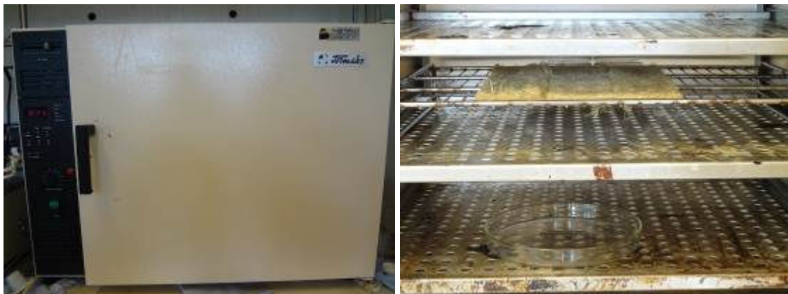
Figure 11: Set-up for applying GMA onto plasma treated hemp non-woven.
