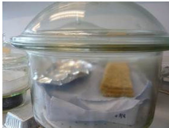
Figure 3: Desiccator to cool pre-dried fibre samples.
