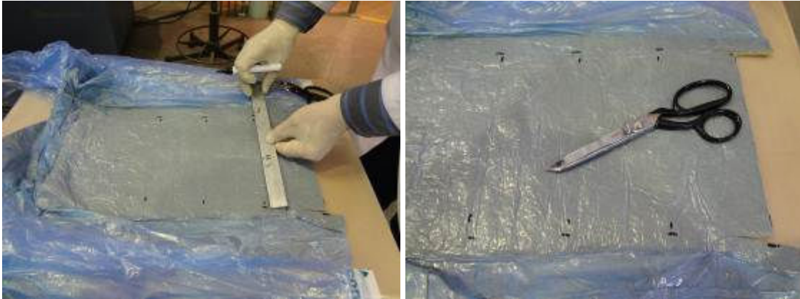
Figure 19: Required SMC sheet dimensions were determined at cut.
