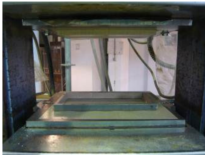
Figure 43: Specially designed mould for lab scale SMC production, fixed in hot press.
