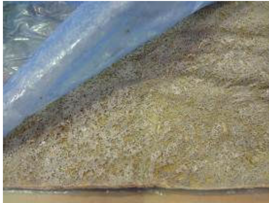
Figure 18: Protecting film released from SMC sheet, showing distribution of resin paste on hemp mat.
