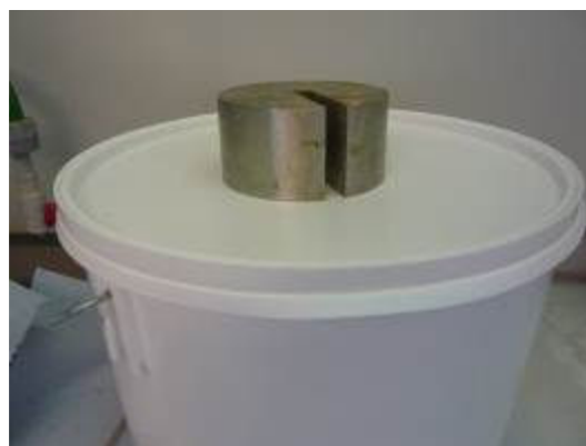
Figure 41: Impregnated fibre samples are matured under 10 kg weight in a closed bucket containing silica gel.
