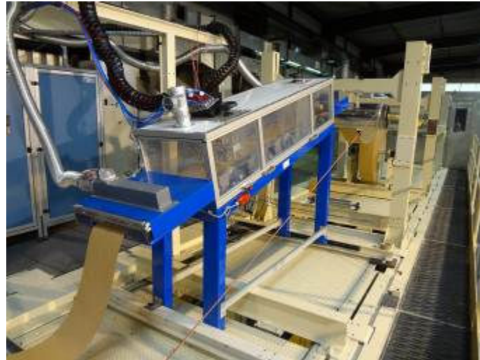
Figure 16: Plasma unit of 25 cm wide used for pilot scale trials.
