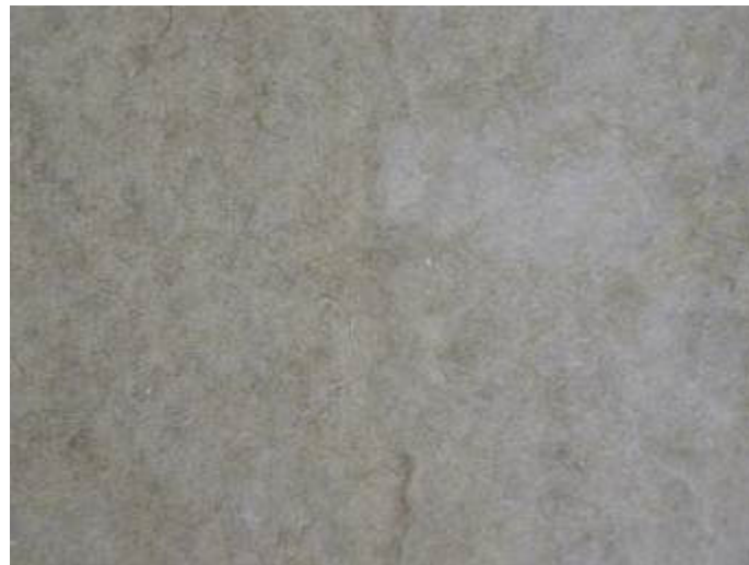
Figure 15: Hemp fibre non-woven produced at Leeds University with (white) Tencel as carrier fibre.
