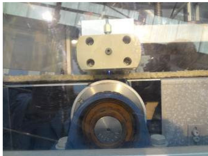
Figure 17: Plasma treatment of natural fibre non-woven.
