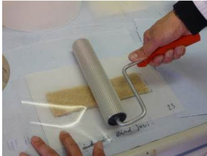
Figure 40: Impregnating fibre non-woven with resin.
