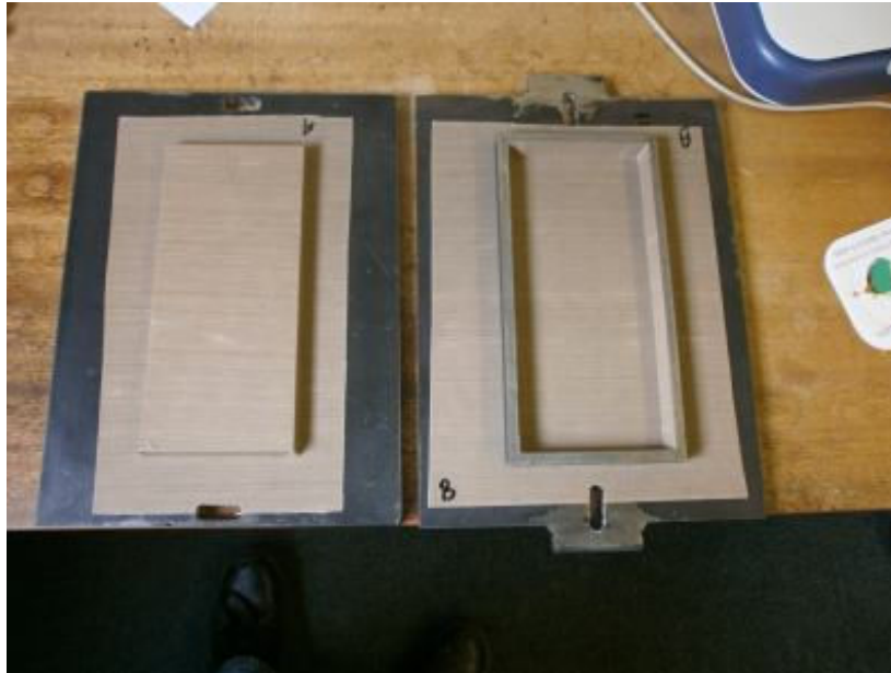
Figure 35: Mould covered with PTFE (Teflon ®) sheets.
