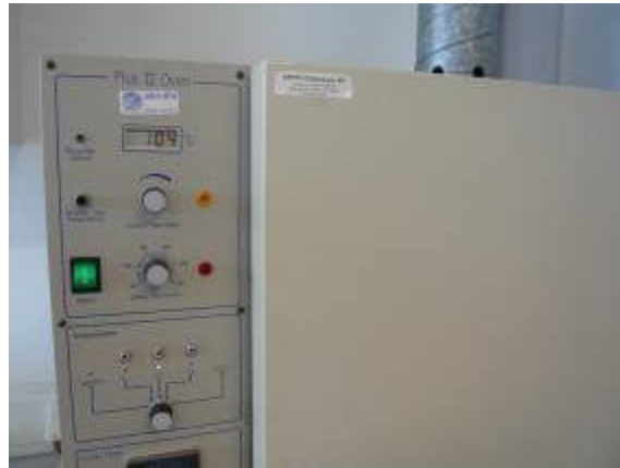
Figure 2: Oven to dry fibre non-woven samples prior to SMC production.
