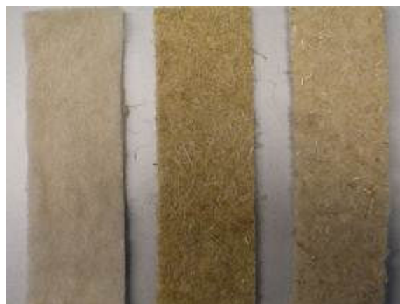
Figure 1: Non-woven fibre samples used for plasma trials: Steam exploded flax (left), needle punched hemp (middle), PLA thermobonded hemp (right).
