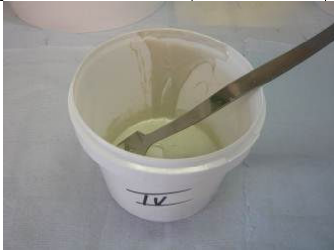
Figure 38: Mixing of resin paste and MgO.
