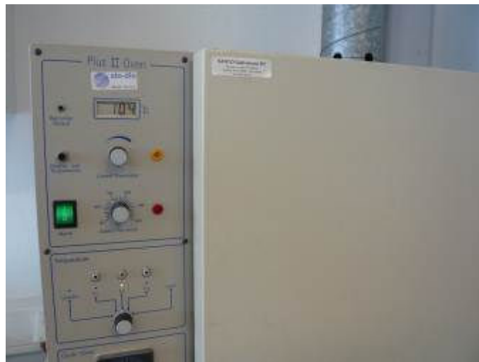
Figure 36: Oven to dry fibre non-woven samples prior to SMC production.
