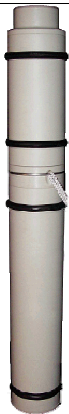
Figure 3: Standard T-POD (taken from www.chelonia.co.uk ); the hydrophone is located at the top, the batteries are stored in the bottom part of the T-POD.
