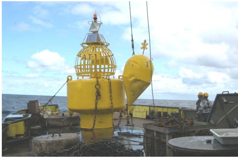
Figure 6. Complete anchoring system on board the “Terschelling” (photo Saskia Mulder, RIKZ)
