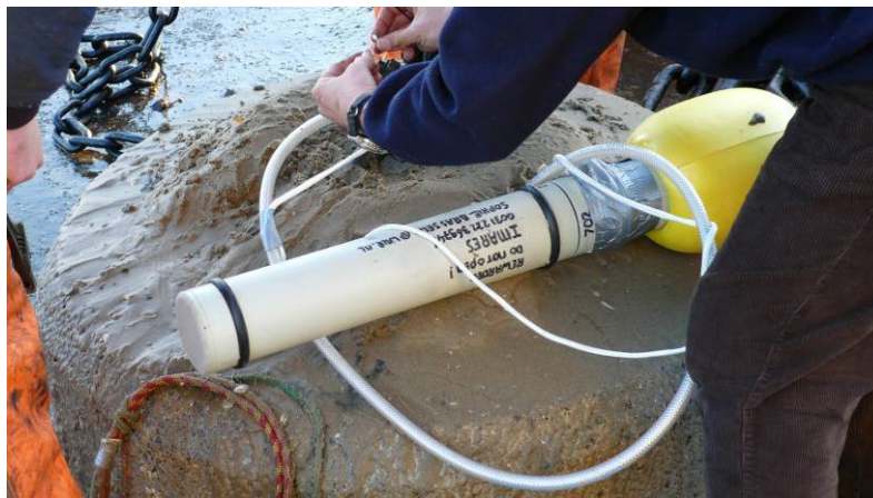
Figure 7: T-POD being attached to the anchoring system. The Kevlar line is reinforced with rubber tubing and a PVC foam float is attached at the top of the T-POD to increase the buoyancy (see appendix 3 for sketch).
