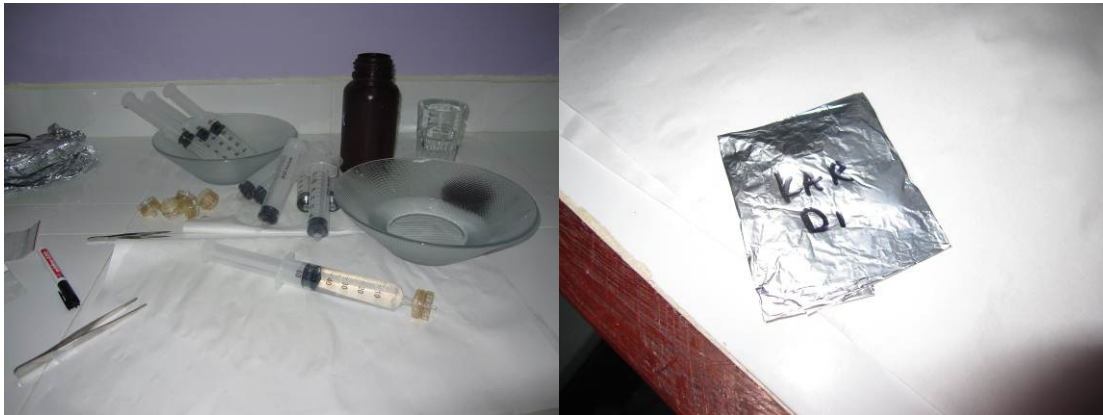
Picture 3. Overview of chlorophyll a processing. Water of 10 syringes with 50 ml were poured through a 0.22 \mu\text{m} filter. The filter is stored in a alufoil for freezing and transport.
