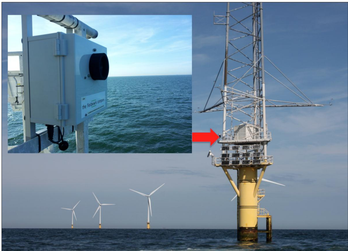
Photo.2 Ultrasonic recorder at the OWEZ wind farm METEO mast. (Photo: Hans Verdaat)
