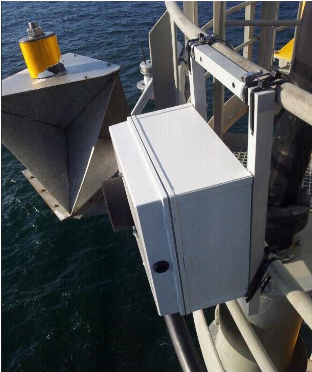
Photo.3 Ultrasonic recorder at the PAWP wind farm WTG 22. (Photo: Andrew Ford)
