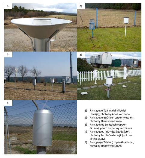
Figure 2.2: Photos of rain gauges in and around the selected catchments.
