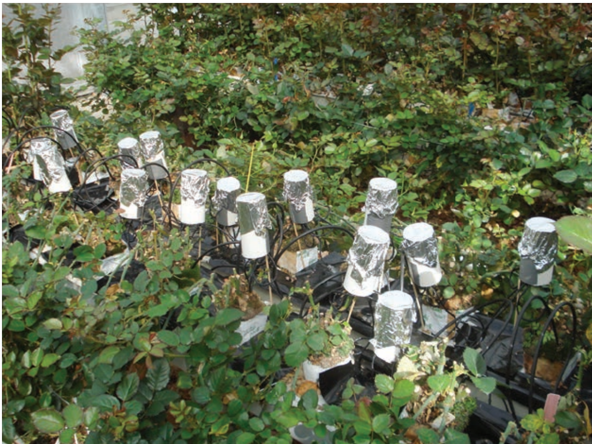
Figuur 3. Lighting tubes. Non-transparent light tubes encapsulating a shoot remainder in rose plants in the experiment on local vs global light (exp. IV). Inside the tubes were LEDs emitting white light.
