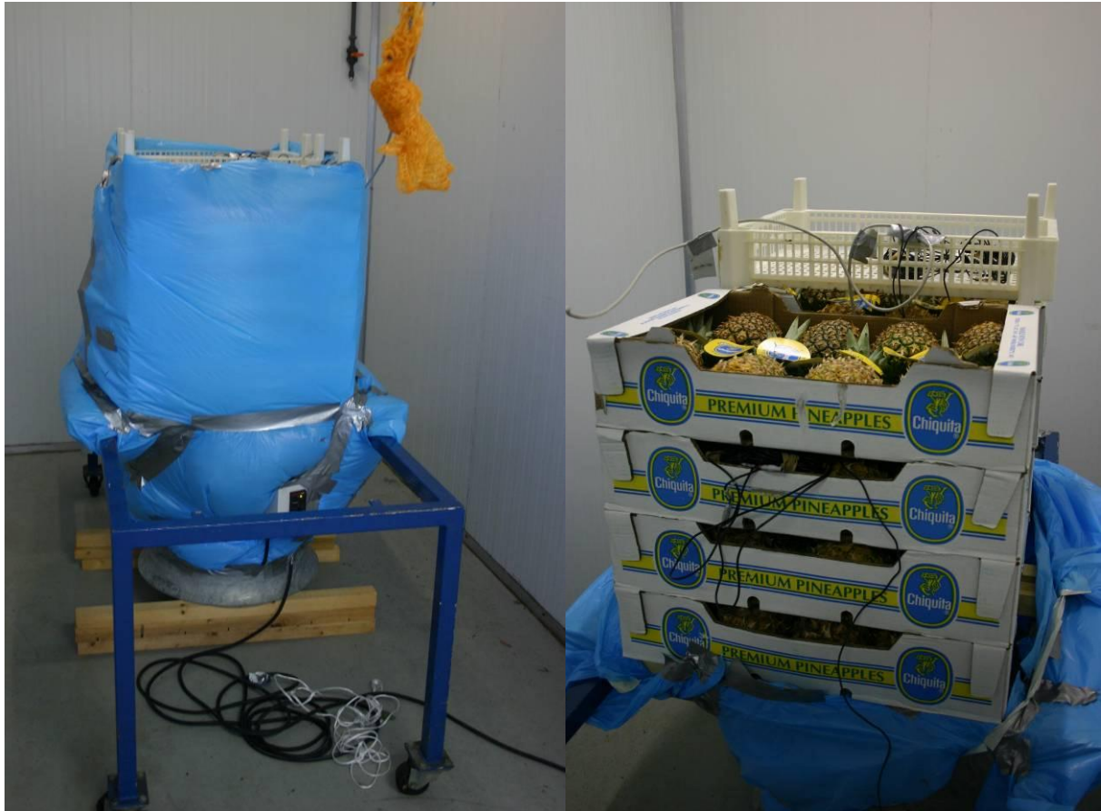
Fig. 9 Experimental set-up at temperature profiles.
