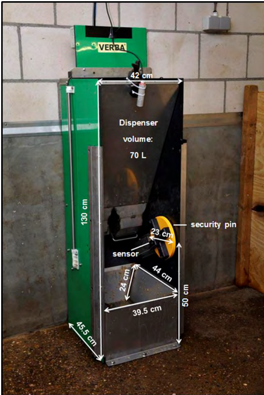
Fig. 3. Tailor-made feeder developed by Verbakel B.V. (Sint Oedenrode, The Netherlands). The feeder was fixed to the wall of the test room, and consisted of a food dispenser, a wheel and a food trough beneath the wheel. By turning the wheel multiple times, the pig would obtain a food reward, which was automatically delivered in the food trough after the required number of wheel turns (detected via the sensor) was performed. Photograph taken by Bart Nijs fotografie.
