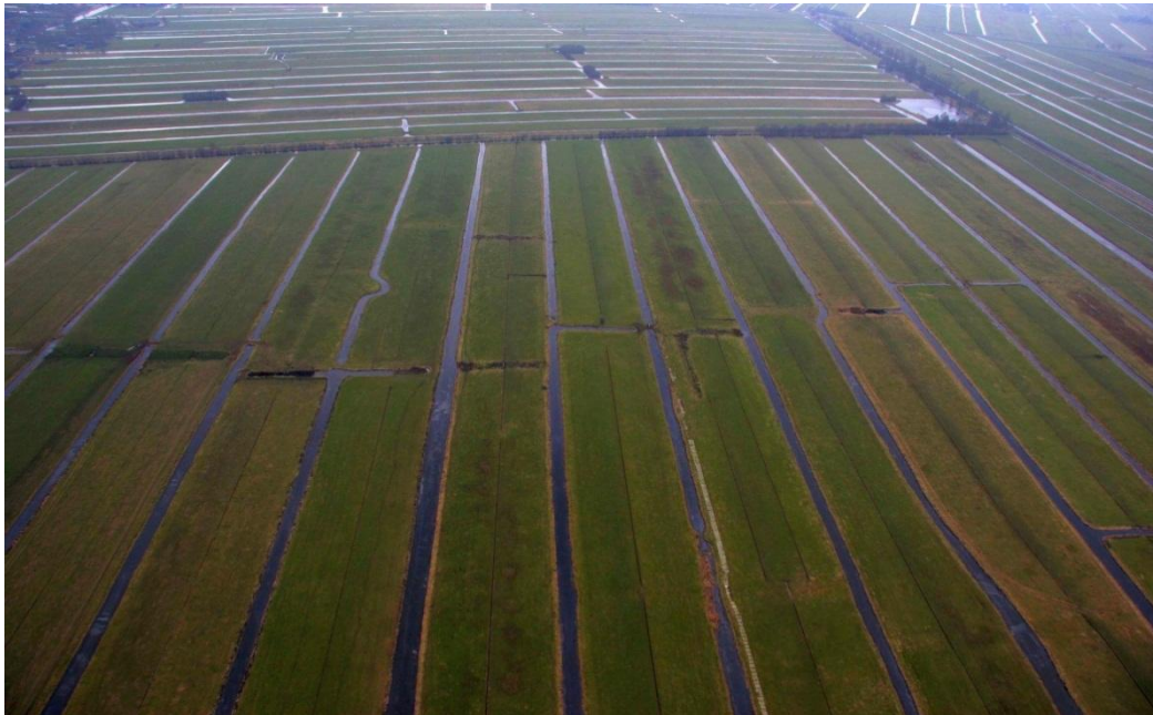
Figure 1. Aerial photo of the typical polder landscape near Kockengen in the Netherlands with a high density of drainage ditches (source: Hoogheemraadschap de Stichtse Rijnlanden)
