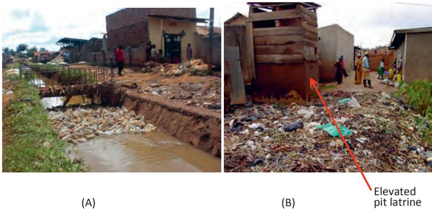
**Figure 3.6: Photographs illustrating sanitation status in Bwaise III in Kampala (Uganda). (A) Blocked storm water drain and (B) Solid waste dump and an elevated pit latrine in the vicinity of a household in a slum area**
