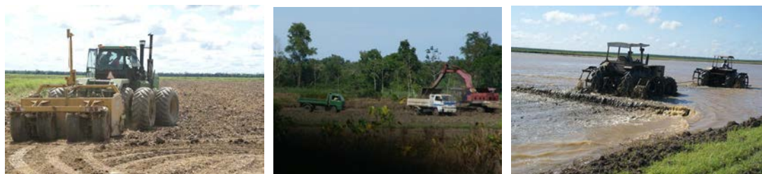
Figure 10 Levelling by scraper (left), hydraulic excavator (centre) both followed by puddling (right).
