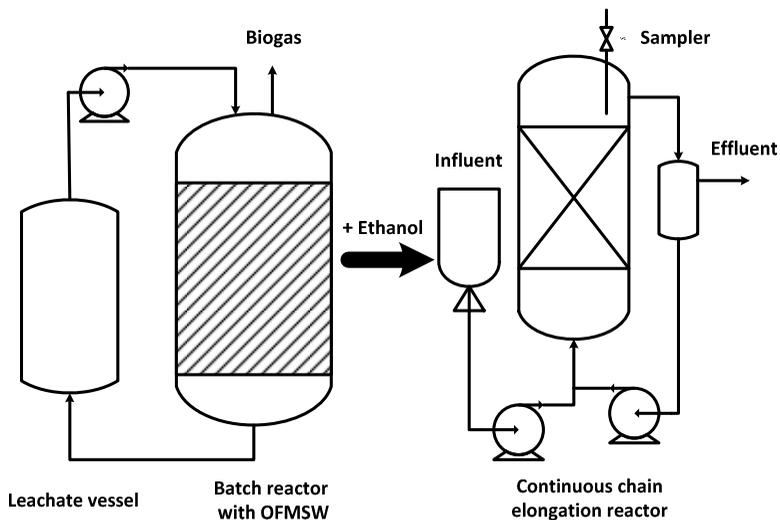
Figure 1. Overview of experimental setup, which consists of an acidification batch reactor to produce VFAs from OFMSW and a continuous chain elongation reactor to produce MCFAs from VFAs and ethanol.
