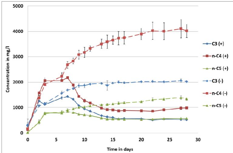
Figure 5. Intermediate product concentrations (propionate (solid diamonds), butyrate (solid squares) and valerate (solid triangles)) clearly decreased after ethanol additions during acidification of frozen waste at 30°C. The dashed lines indicate the intermediate product concentrations in the control experiment without ethanol additions.
