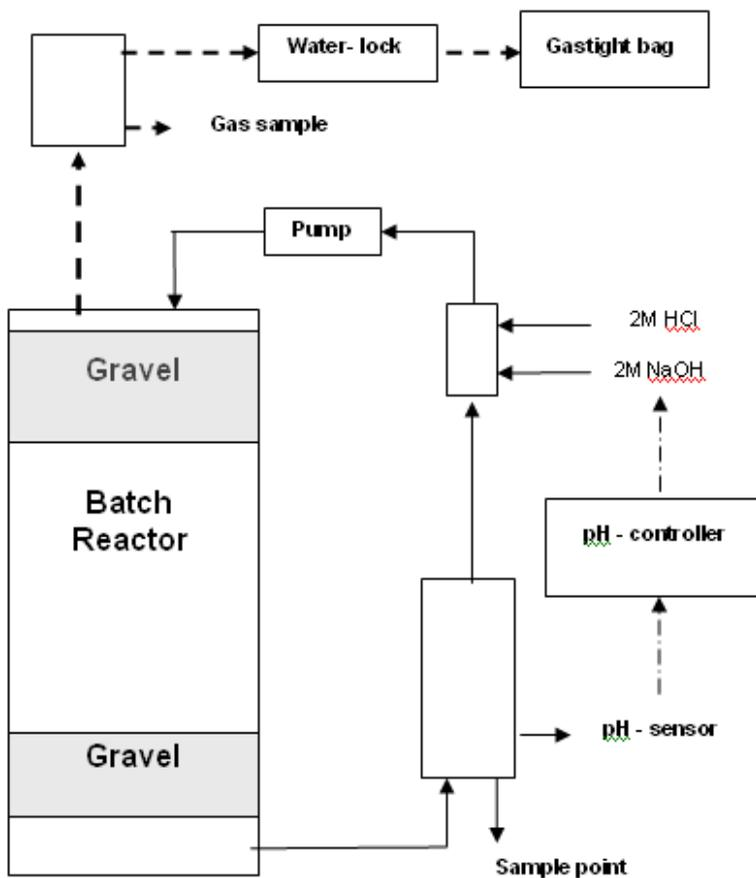
Figure 1. Experimental set-up of the reactors. Solid lines represent liquid streams, while the dashed lines stand for gas streams. The dash-dotted lines are signals to and from the pH-controller.
