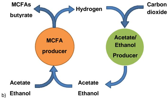
Figure 2a,b. Possible interactions between carbon dioxide based hydrogen scavengers and MCFA producers. If hydrogen is consumed by acetate/ethanol producers (b), additional substrate for chain elongation could be produced from carbon dioxide.
