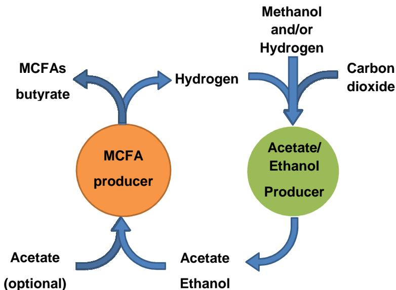
Figure 3. Possible consortium to replace ethanol with methanol and/or hydrogen/carbon dioxide
