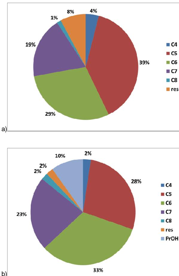
Figure 2 a,b. Increasing the ethanol load leads to higher heptanoate (C7), caproate (C6) and propanol (PrOH) selectivity at expense of mainly valerate (C5) selectivity. Figure 2a shows the product selectivity during phase II (propanol was not measured in that phase). During phase III (Figure 2b), a higher ethanol load was applied.
