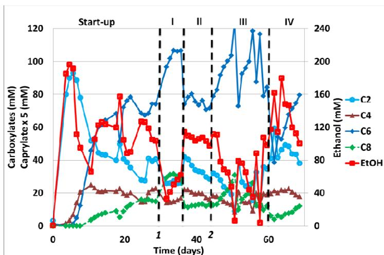
Figure 1. Concentration overview of carboxylates and ethanol during experiment. At 1 (day 32) the  $\text{K}_2\text{CO}_3$  concentration was increased to  $8.0 \text{ g l}^{-1}$ , while at 2 (day 45) the yeast extract concentration was doubled. Acetate concentrations are given by open circles, ethanol by open squares (right y-axis), butyrate by closed triangles, caproate by closed diamonds and caprylate by closed diamonds with dashed lines.
