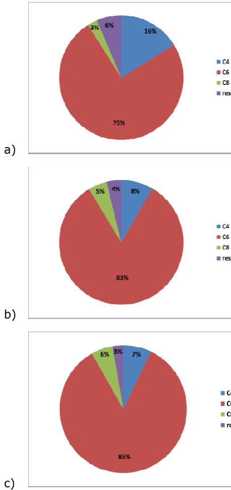
*Figure 4. Distribution of product formation during phase I (a), phase II (b) and phase III (c) based on consumed electrons from acetate and ethanol. Increasing the ethanol load leads to more selective MCFA production (C6+C8), while butyrate production (C4) and other residual products (res), including biomass, are reduced.*
