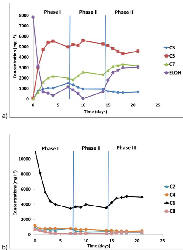
Figure 1a,b. Concentration overview of carboxylates and ethanol during experiment. Odd numbered carboxylates and ethanol (C3, C5, C7 and EtOH) are presented in the upper figure (1a), while even numbered carboxylates (C2, C4, C6 and C8) are presented in lower figure (1b). Besides heptanoate (C7), mainly valerate (C5) and caproate (C6) are produced.
