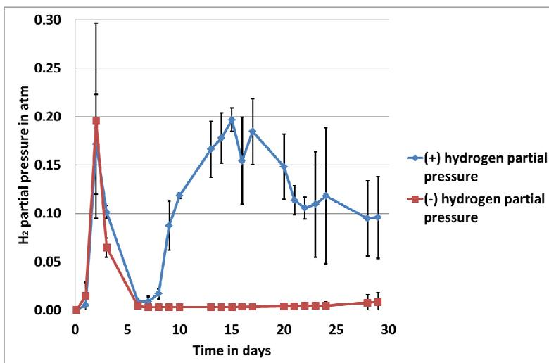
Figure 3. Hydrogen partial pressures during experiments with frozen waste.
