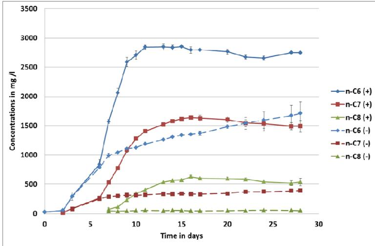
Figure 4. After ethanol additions, caproate (solid diamonds), heptanoate (solid squares) and caprylate (solid triangles) concentrations increased clearly during acidification of frozen waste at 30°C. The dashed lines indicate the MCFAs concentrations in the control experiment without ethanol additions.
