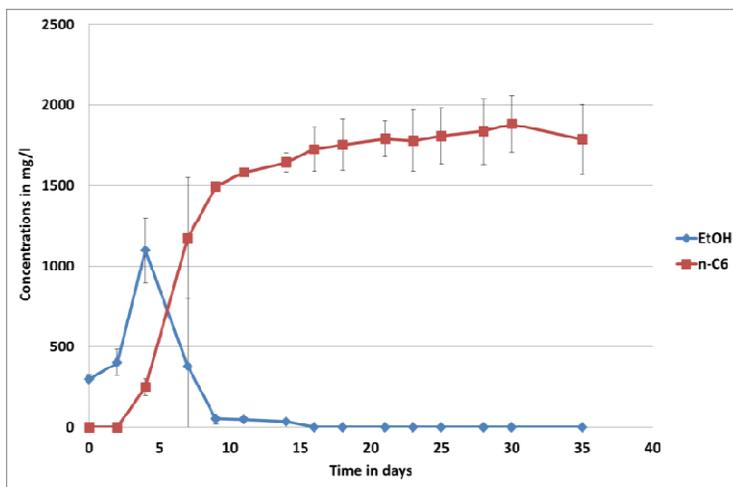
Figure 1. During acidification of fresh waste at  $30^{\circ}\text{C}$ , caproate formation (squares) and ethanol formation (diamonds) were observed. Most of the caproate formation coincided with ethanol degradation from day four until day nine, indicating that caproate is formed from ethanol.
