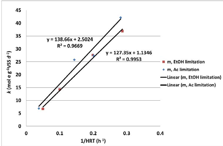
Figure 2. Tempest plots of *C.kluyveri* (based on data of Kenealy and Waselefsky (1985)) provide information to estimate the maintenance coefficient.
