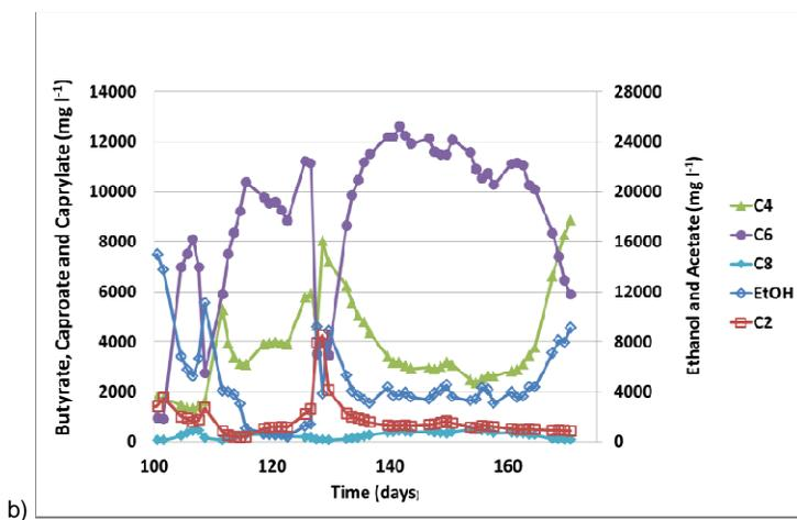
Figure 2. Overview of experimental results (chain elongation reactor) in the complete experiment (a) and the experimental results of period III (after installing the pH controller on day 102) (b).
