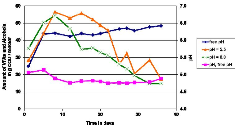
Figure 2. Comparison of total intermediate production in leachate for three pH conditions.
