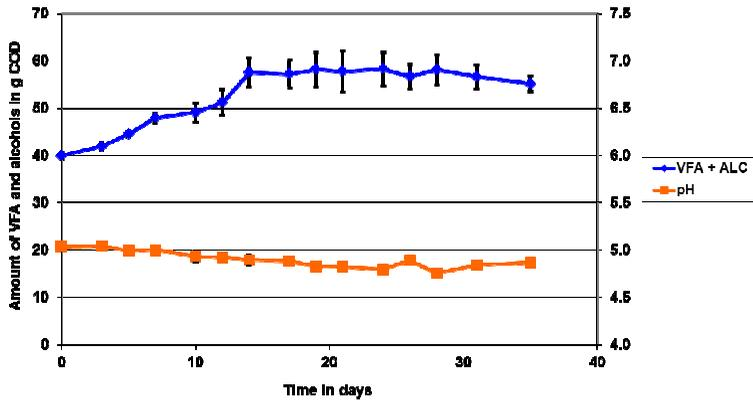
Figure 3. The second experiment confirmed that large acetate consumption could be prevented in a dry anaerobic reactor without pH control.
