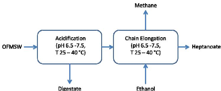
*Figure 4. Schematic overview of the two-stage heptanoate production process.*
