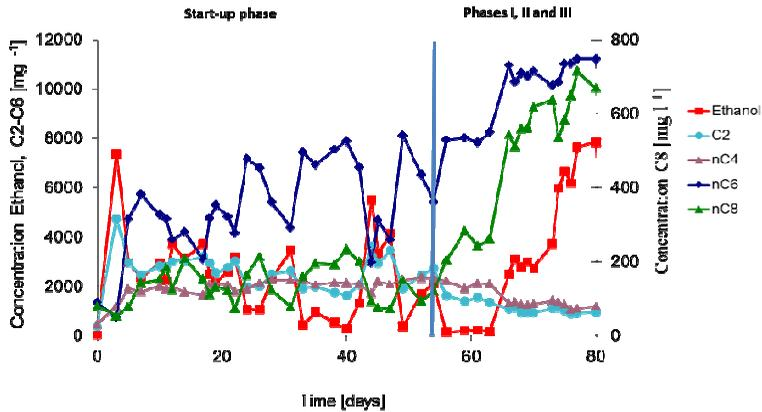
Figure 2. Results of the whole experiment, which can be divided in a non-stable period, the start-up phase, and a stable period including phases I, II, III. The start-up phase could not become stable due to pH variations and clog-ups. From day 55 on stable reactor operation was achieved with high MCFA production. The concentrations of ethanol, acetate (C2), butyrate (nC4) and caproate (nC6) are displayed on the left axis, while the concentration of caprylate (nC8) is displayed on the right axis.
