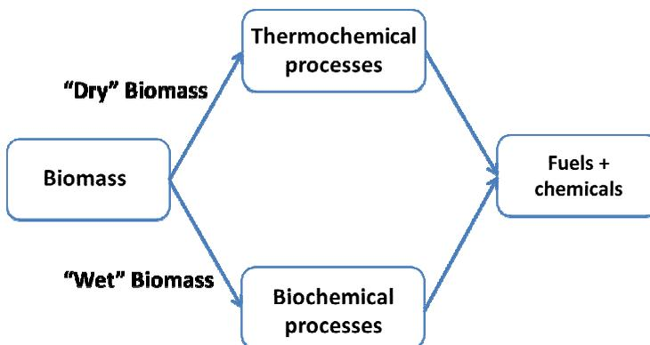
Figure 2. Biomass can be converted by thermochemical processes and biochemical processes to fuels and chemicals. “Dry” biomass refers to biomass with a water content lower than 30 wt%, while “Wet” biomass is defined as biomass with a water content lower than 70 wt%.
