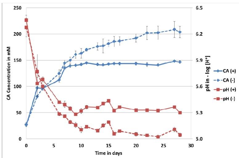
Figure 6. The total carboxylic acid ( $CA = \sum C2-C8$ ) production during acidification with ethanol addition (solid diamonds) is significantly lower than the total carboxylic acid (CA) production without ethanol additions (dashed diamonds). As result, the pH is higher in reactors with ethanol additions (solid squares) than in the reactors without ethanol additions (dashed squares).
