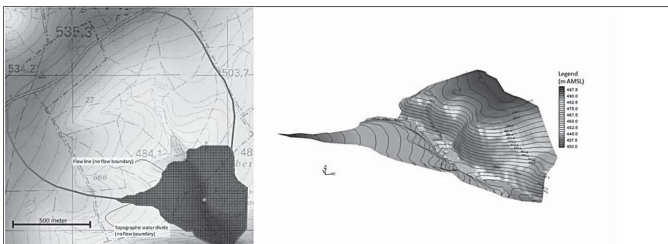
Figure 5: a) Topographical map with elevation, catchment boundary (grey line), model area (black grid) and gravimeter location (green dot), and b) three-dimensional image of the surface level of the modelled area
