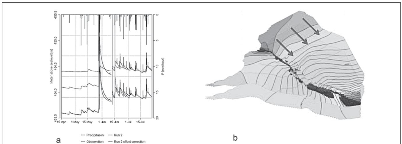
Figure 6: Model results as a) measured and simulated groundwater levels underneath gravimeter (2007) and b) transient simulated groundwater flow
