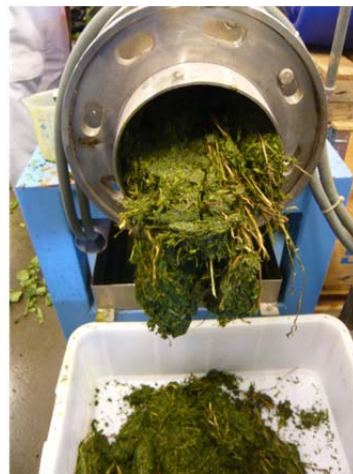
Figuur 5: Clextral BC45 Twinscrew extruder
