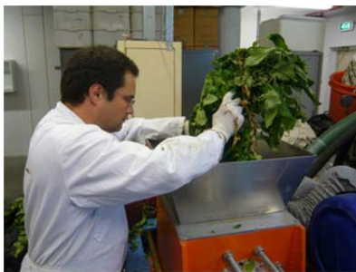
Figuur 5: Clextral BC45 Twinscrew extruder
