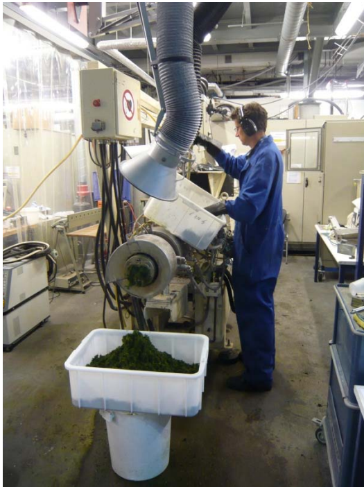
Figuur 5: Clextral BC45 Twinscrew extruder
