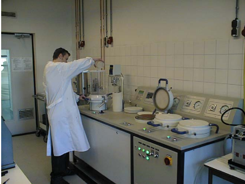
Figuur 10: Rapid Köthen sheet former
