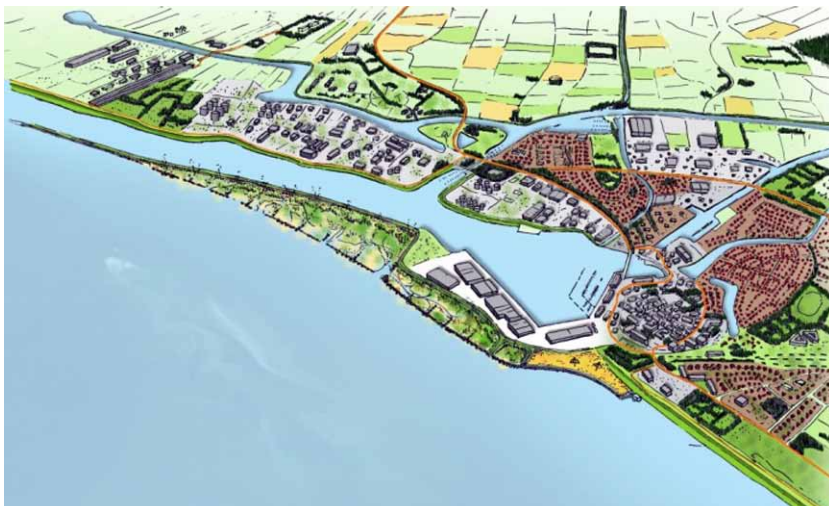
Figure 6 An artificial saltmarsh design using sediments from the nearby harbour.
