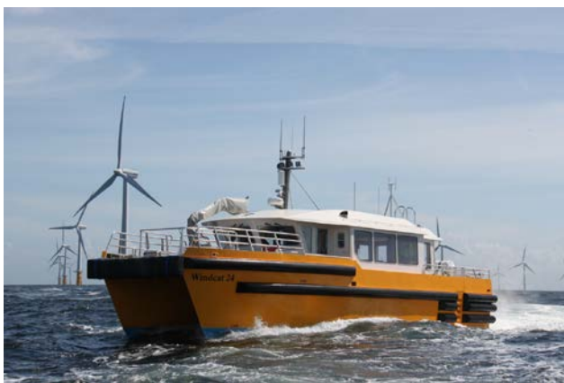
Figure 8 Catamaran vessel (type “WindCat”) used to transfer personnel for maintenance and repair to wind turbine terminals (particulars: Design 2010, constructed of aluminium. Dimensions: length overall 18.0 m x width 6.1 m x depth 1.8 m. Main engines 2 x MTU V8, 960 HP each with Servogear gearboxes. Propulsion 2 x Servogear variable pitch props with Scanmar controls).
