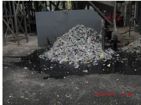
Figure 44: Discharged light by-products.
