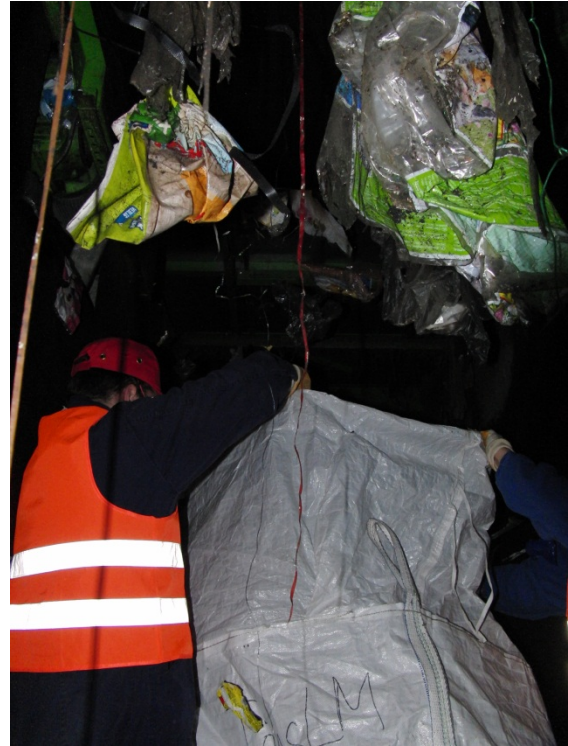
Figure 31: Obtaining a sample from the mixed plastics fraction in the bunker in Kempen.
