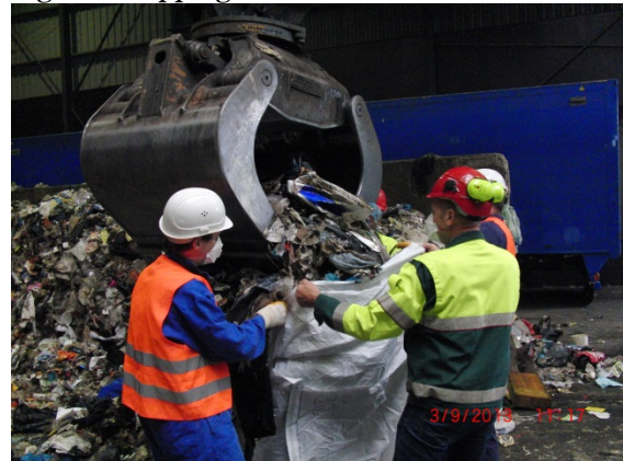
Figure 12 Obtaining a grab sample using the excavator
