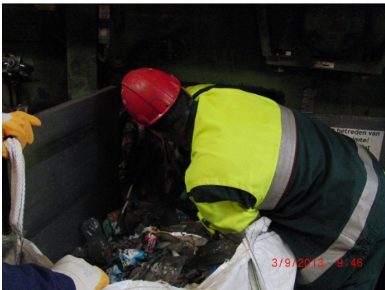
Figure 10 Cleaning of the chamber of the press for the plastic and beverage carton mix
