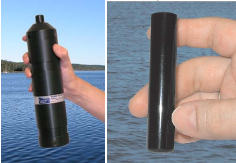
Figure 14. Left: VEMCO VR2W-69 kHz acoustic receiver. Right: VEMCO V16 coded transmitter [ http://vemco.com/ ]
