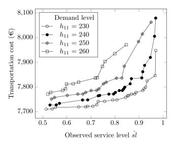
Figure 3.2: Minimum transportation cost fulfilling demand  $h_{11}$  at service level  $\hat{sl}$ .
