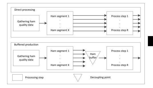
Figure 2.2: Schematic overview of buffered and non-buffered process design scenarios.
