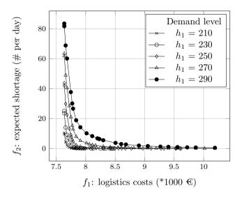
Figure 4.2: Pareto fronts obtained using the weighting method procedure for variations of  $h_1$ .
