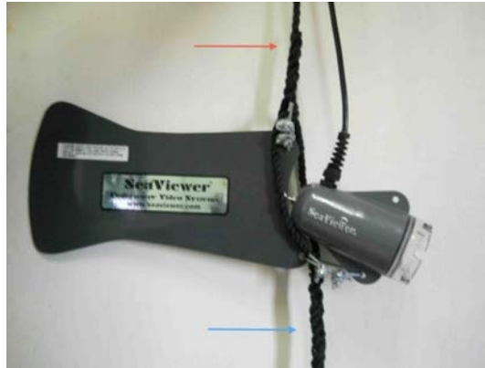
Figure 2. Attachment of the rope to the camera. The red arrow points to the safety line, the blue arrow points to the weighted line.
