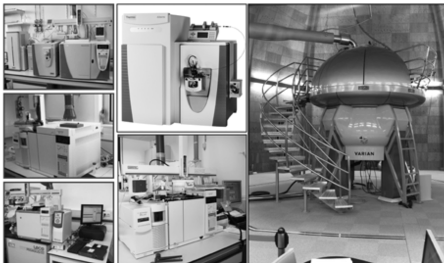
Figure 4. Metabolomics application is centred around the use of advanced, state of the art equipment such as mass spectrometers (left and middle) and NMR machines (right).
