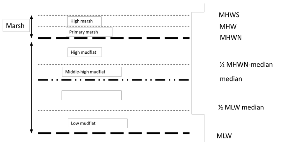
Figure 4.11 An overview of the position of intertidal habitat types with respect to sea level (median). MLW=Mean Low Water, MHW= Mean High Water, MHWN= Mean High Water Neap tide, MHWS=Mean High Water Springtide (Soresma 2009)(translated).
