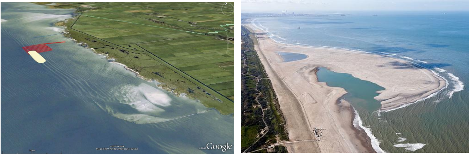
Left: Impression of a nourishment in Lake IJsselmeer near Workum; right: the sand engine in front of the Dutch coast.
