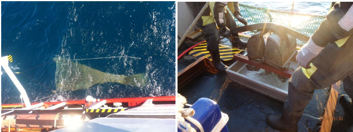
Figure 2. Deployment of the two meter beam trawl (left) and the van Veen grab (right).
