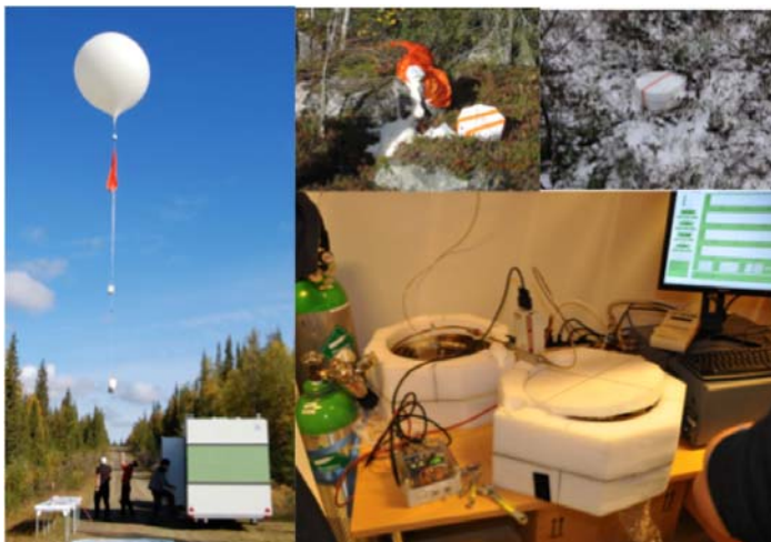
The launch(left), the recovery from the field (top right), and the analysis of AirCore in the laboratory (bottom right).
