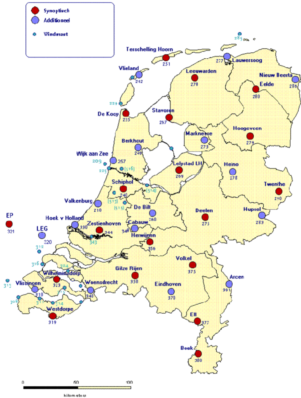
The land part of the synoptic network of the Netherlands. Red dots are the main stations. The large blue dots are the additional stations, and the small blue dots are wind mast.
