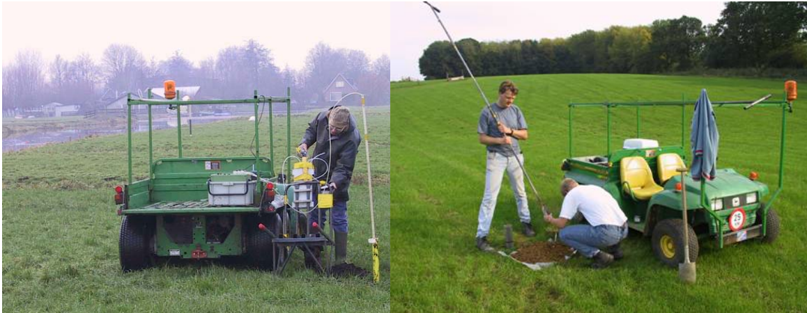
Figure: 2.2 Sampling of the uppermost metre of the groundwater on peat soil (left) and soil moisture sampling on loess soil (right).
