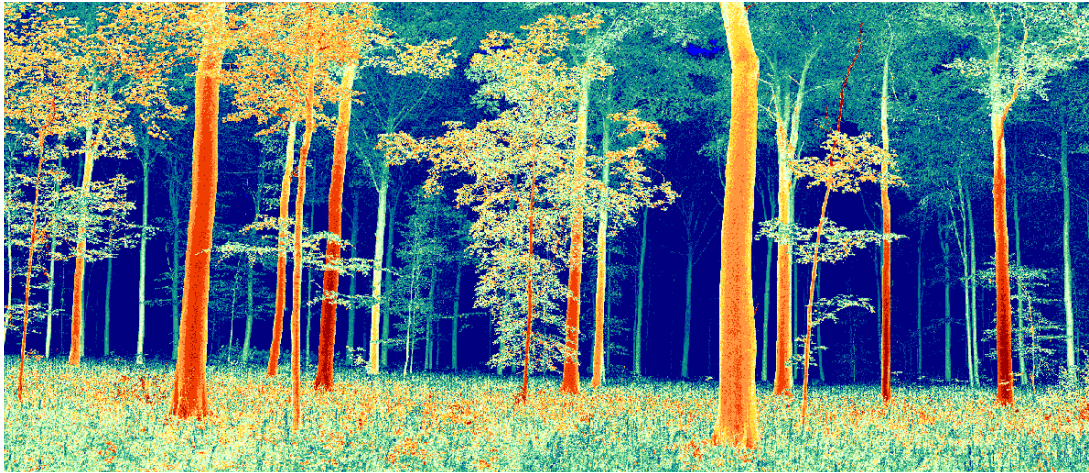
Figure 1.1: Illustration of terrestrial LiDAR data in a cylindrical projection. The data was captured in a Hallerbos (Belgium) and coloured according to returned intensity (blue is low intensity, red is high intensity).
