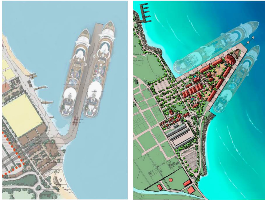
Fig. 4. (a) The finger pier design. Adapted from: [22]. (b) The peninsula design. Adapted from: [20].
