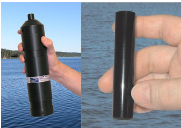
Fig. 2. Vemco receiver (left) and V16 transmitter (right) (photo's Vemco)
