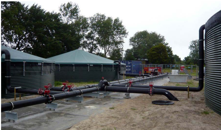
Figure 1 The IMARES test facility where the tests were performed, with on the right the 730 m 3 feed tank and on the left the two 250 m 3 test tanks
