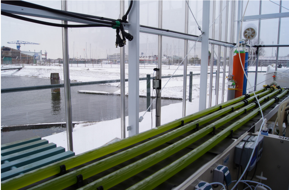
Fig. 3 Pilot-scale horizontal tubular photobioreactor in the SEA Lab of HZ University of Applied Sciences in Vlissingen, the Netherlands.
