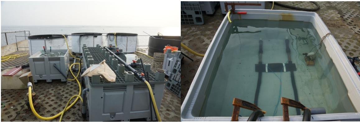
Figure 6. Overview of the holding tanks and the exposure tank equipped with the HFK electrodes
