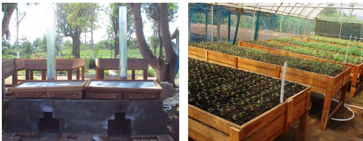
Figure 5. The build soil steamer to disinfect substrates (left) for the mini-tuber production at Heho (right) (Holdinga et al. 2014).
