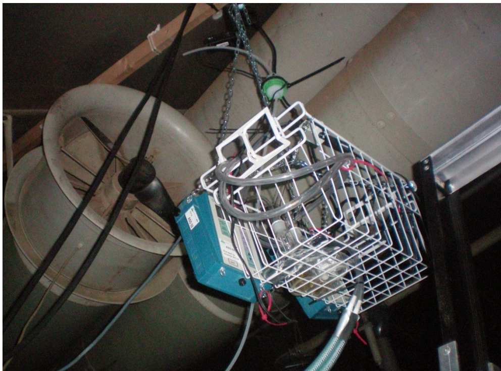
Figure 1 Air outlet in the room with fattening pigs and the installed measuring equipment.
