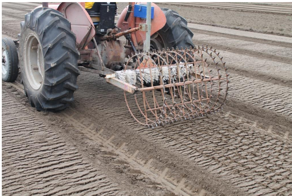
Figure 6 Current machinery used to dibble the planter beds with tearing visible
