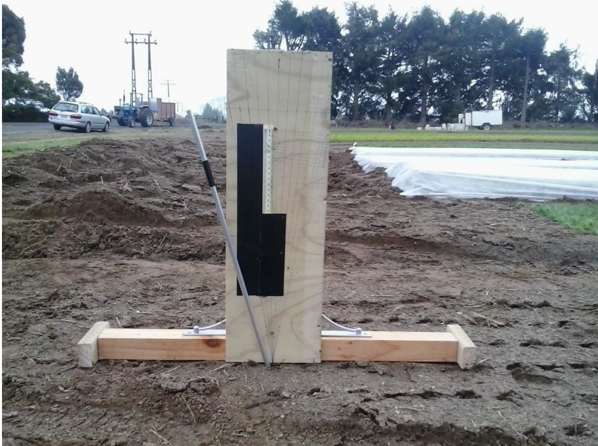
Figure 18 Measuring depth and angle of hole made by spiked wheel dibbler
