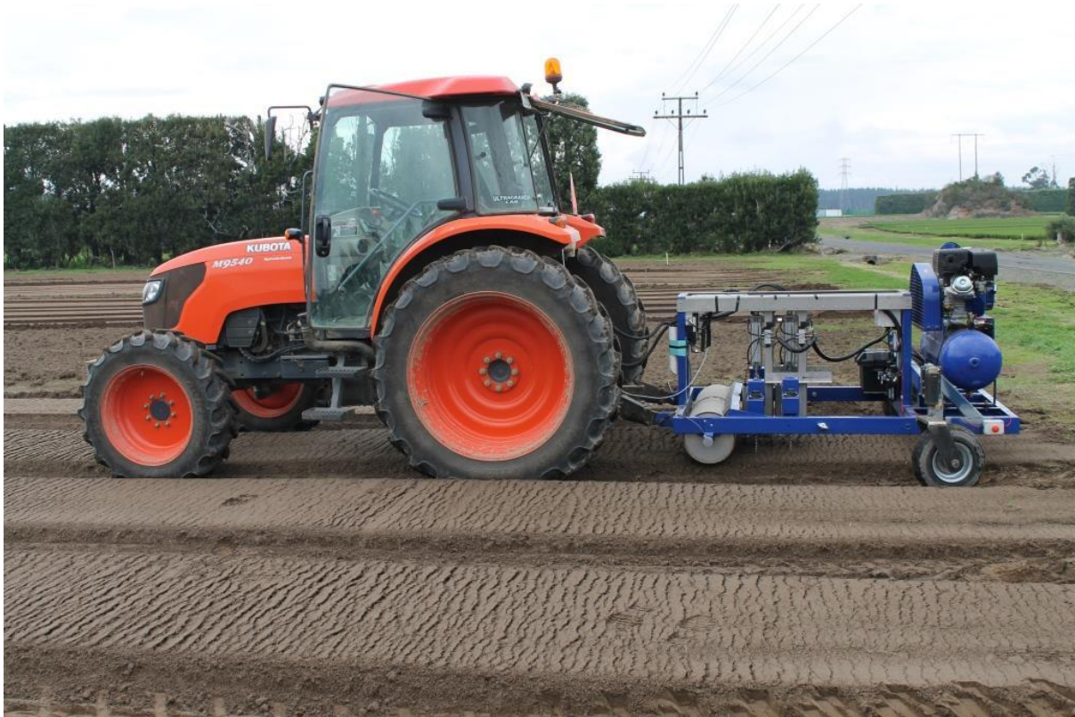
Figure 15 New dibbler and tractor
