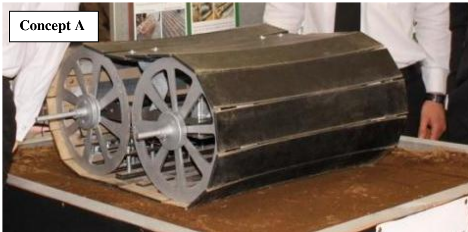
Figure 9 Caterpillar tracked dibbler mock-up
