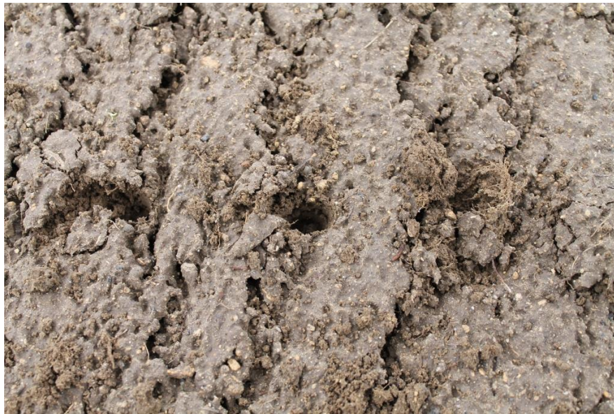
Figure 7 Plan view of the holes produced from the current dibbling machine
