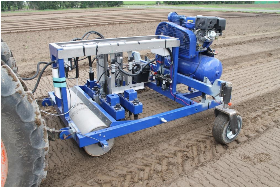
Figure 14 Finished machine dibbling holes at the nursery
