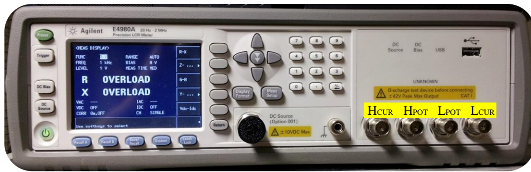
Figure 3-3: Measurement terminals of Agilent E4980A auto balancing bridge instrument
