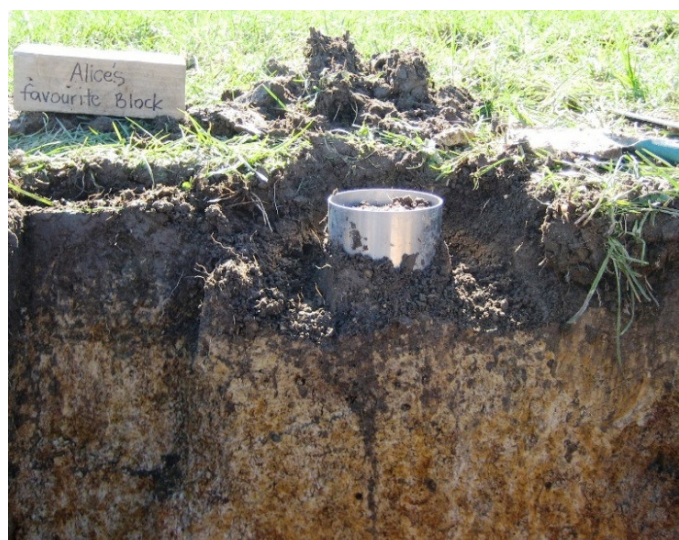
Figure 3.6. An example of a soil dry bulk density core being carved in to an A horizon
