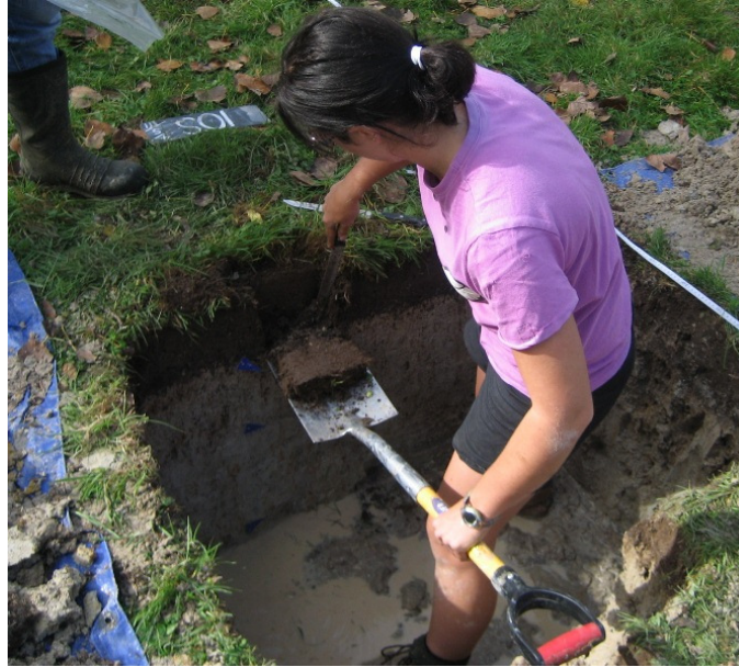
Figure 3.5. An example of a slice of an A horizon being taken for total C and N analysis.
