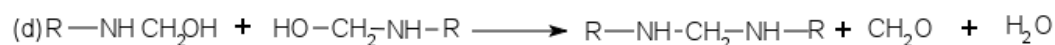
Figure 1.8 The reactions of methylol with amino, imino and other methylol groups where R is the melamine moiety. Adapted from reference 9.
