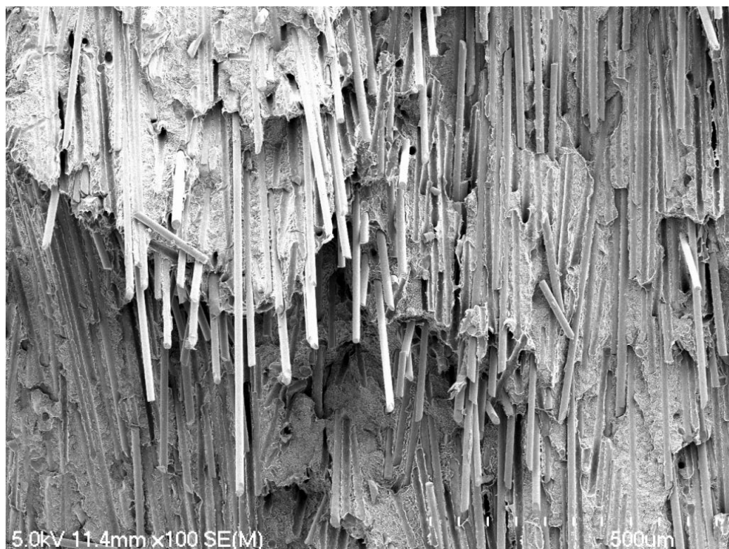
Figure 4.32: SEM image of the fracture surface of a rotomoulded HMA-018 HDPE / glass fibre sample, produced from granules with dimension of approximately 1.5mm x 4mm.
