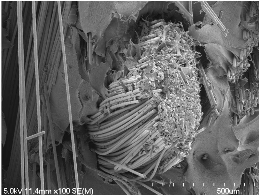
Figure 4.17b: SEM image of the fracture surface on a “dry-mix” Vanglobe 8539/glass fibre composite impact-test specimen.
