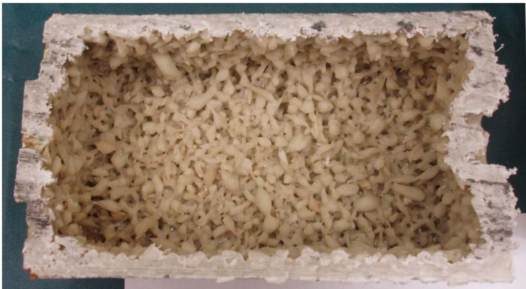
Figure 4.6: The poor rotomoulding granule coalescence seen with the Cotene 9800 PP/glass fibre composite.
