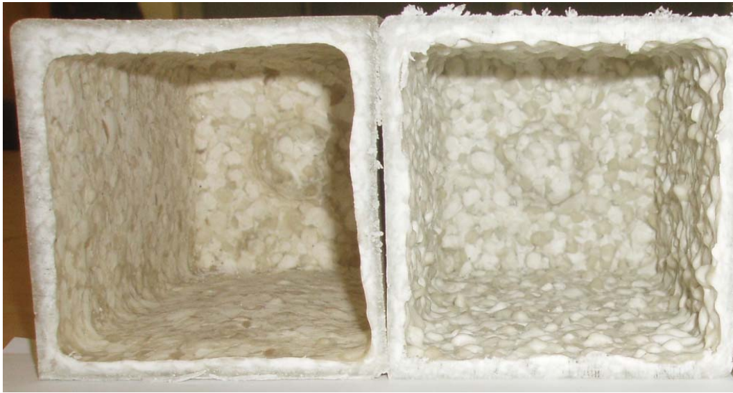
Figure 4.13: Rotomoulded samples produced from HP741T polypropylene-matrix composite granules, containing 10vol% glass fibre (left) and 20vol% glass fibre (right).
