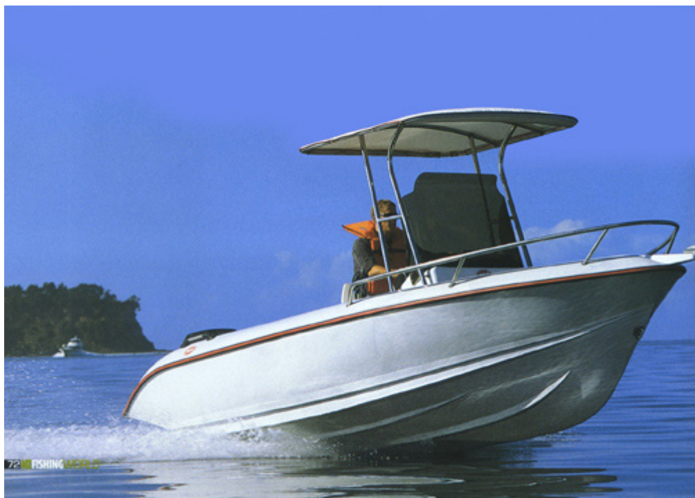
Figure 1.2: Example of a rotationally moulded product - The outer hull of this Galloway International Ltd Mac boat is a one-piece polyethylene moulding [8].
