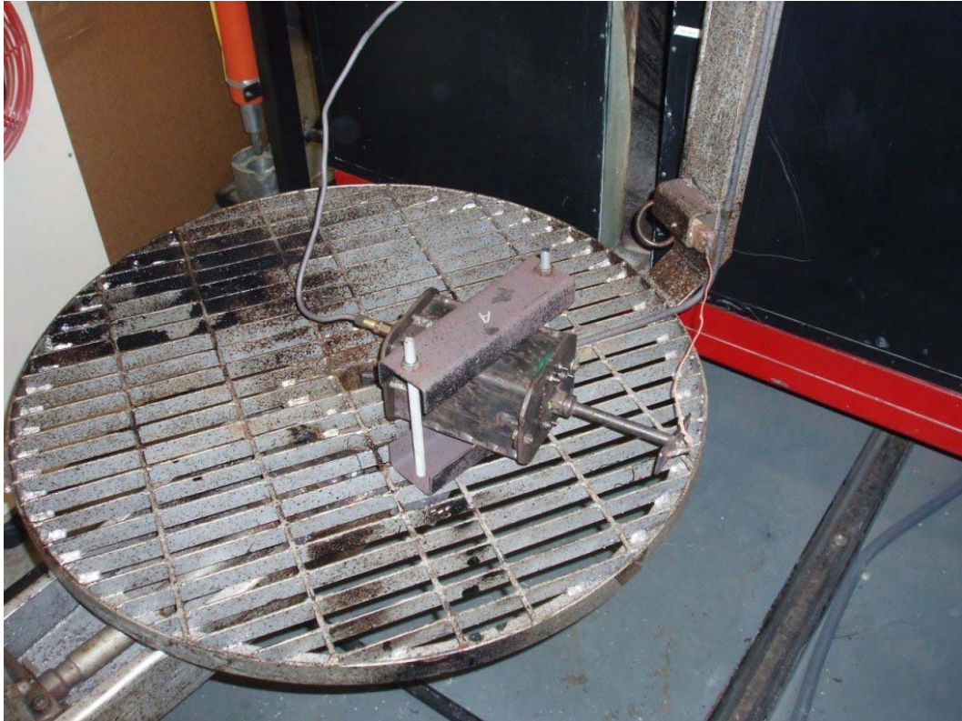
Figure 3.4: The small sample-mould fitted to the turret of the R&D system rotational moulding equipment.
