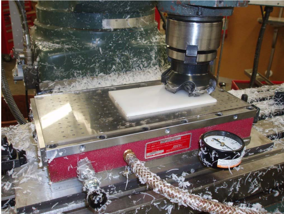
Figure 3.10: Milling a polymer sample sheet to a controlled thickness. The sample is retained in place by vacuum.
