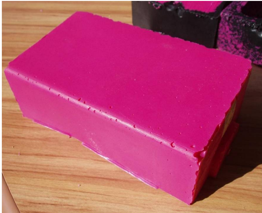
Figure 4.3: Single-shot rotational moulding from granulated Cotene 3979 HDPE.
