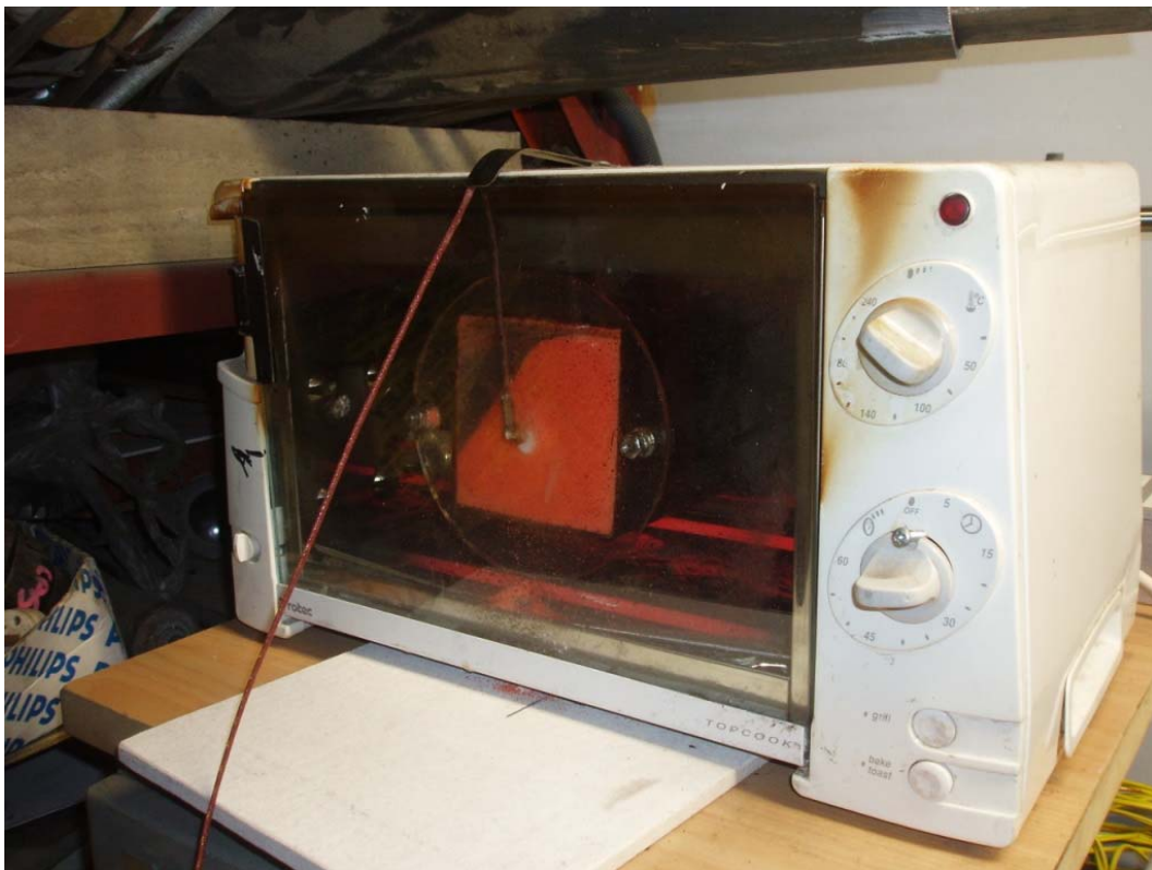
Figure 3.2: The "micro-oven" rotational moulding apparatus.
