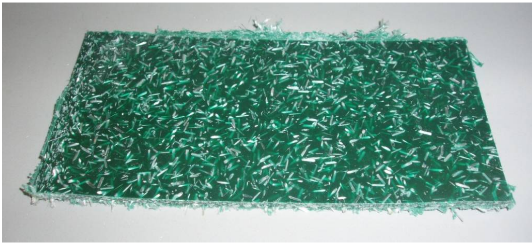
Figure 4.16: Typical fibre distribution in a rotationally moulded “dry-mix” polyethylene/glass fibre composite.
