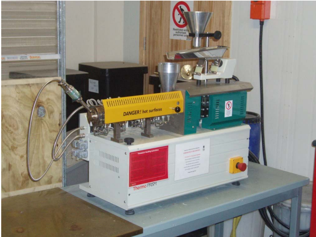
Figure 3.1: The ThermoPrism TSE-16-TC extruder used over the course of this research.
