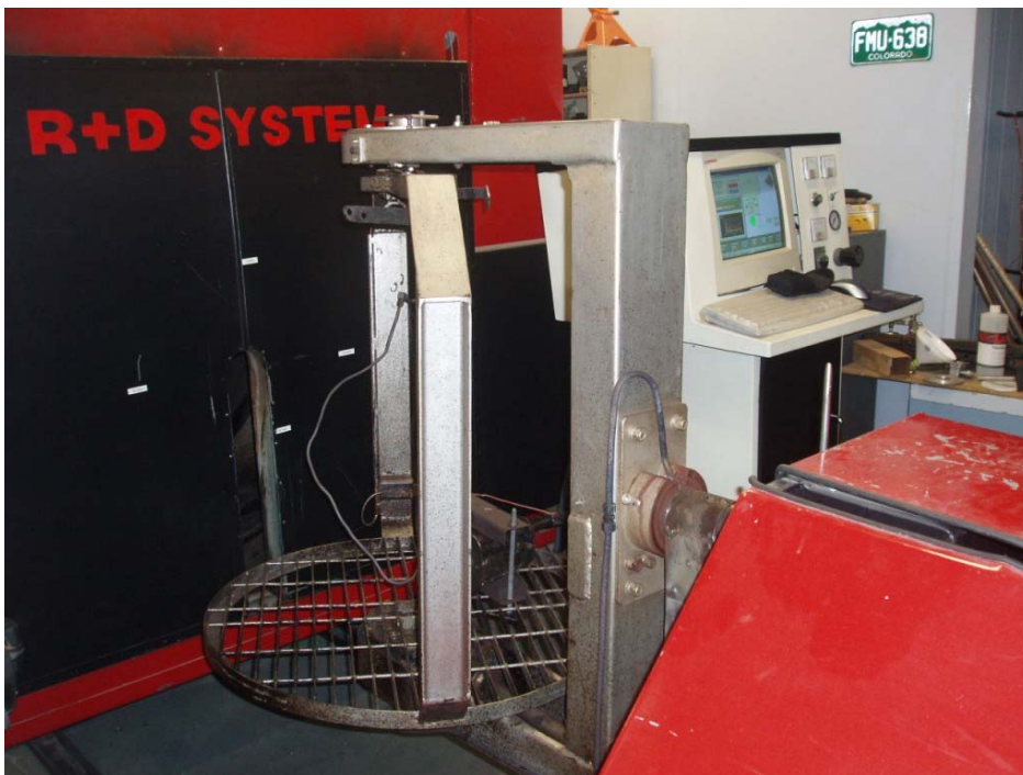
Figure 3.3: The “R&D System” rotational moulding setup
