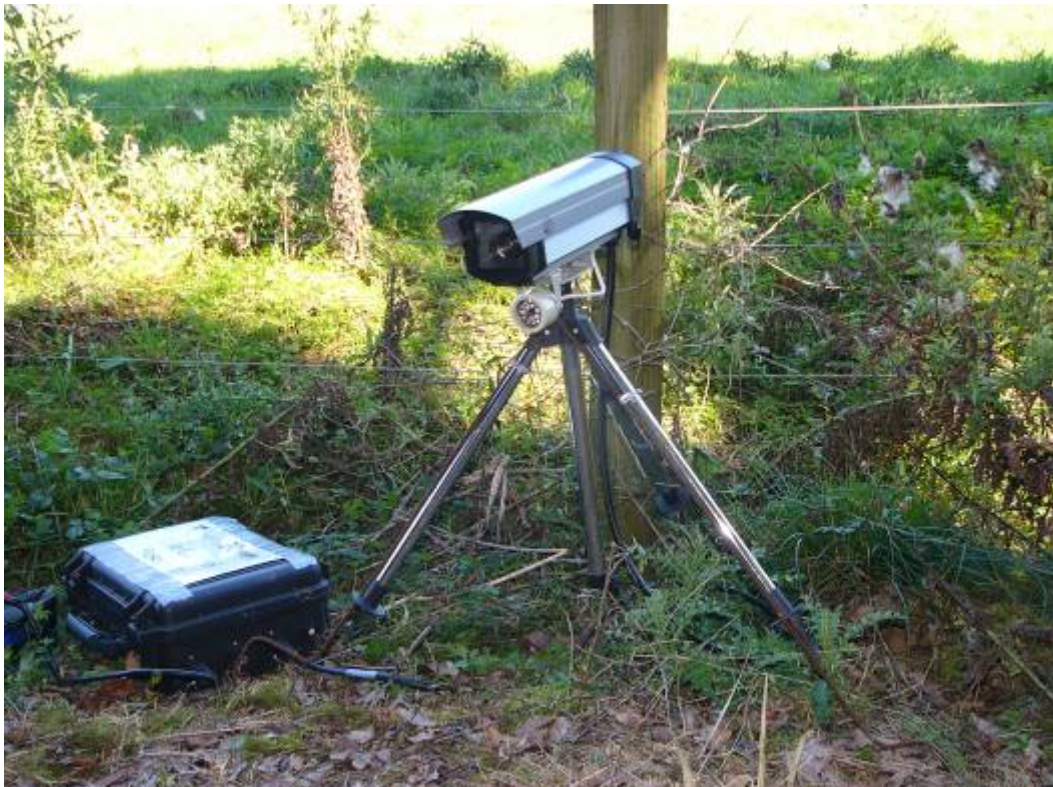
Figure 7. A video camera, infra-red light and video recorder (in black case), set up opposite a simulated breach.
