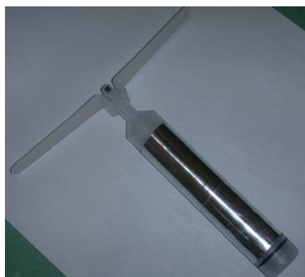
Figure 4.15. PP EMID covered in tinfoil showing a window along the length of the EMID in the tinfoil to allow the piston to be seen.
