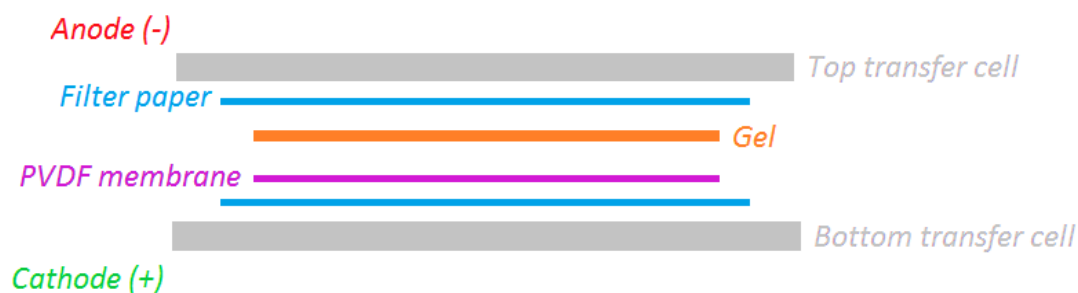
Figure 51. Layout of semi-dry transfer for Western blotting.
