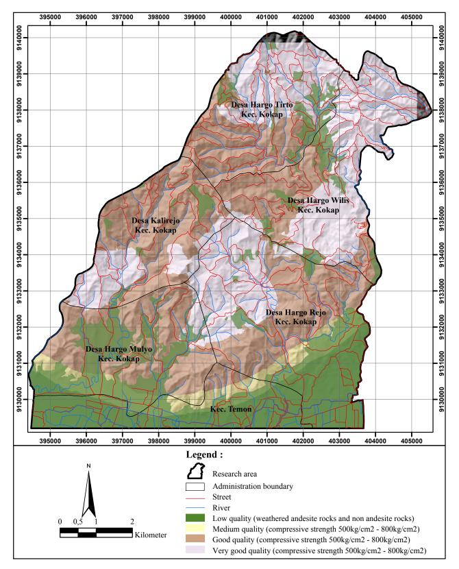
Figure 5: Distribution of andesite rocks quality (classification based on compressive strength requirements of rocks for building foundations and road according to Keputusan Meneri Pekerjaan Umum Nomor: 306/KPTS/1989, SK SNI S-04-1989-F).
