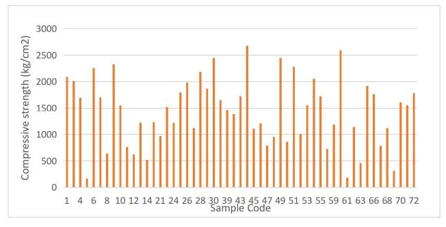
Figure 3: The compressive strength value of the testing samples taken from igneous rock intrusions in the study area.
