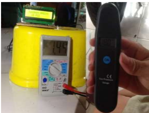
Figure 9. (c). The results of the comparison between the TPMS Prototype and the Digital Tire Pressure Gauge Tool worth 18 PSI
