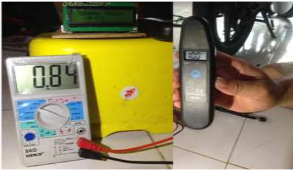
Figure 9. (a). The results of the comparison between the TPMS Prototype and a 10 PSI Digital Tire Pressure Gauge Tool
