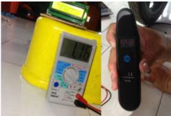
Figure 9. (b). The results of the comparison between TPMS Prototype and Digital Tire Pressure Gauge Tools worth 15 PSI
