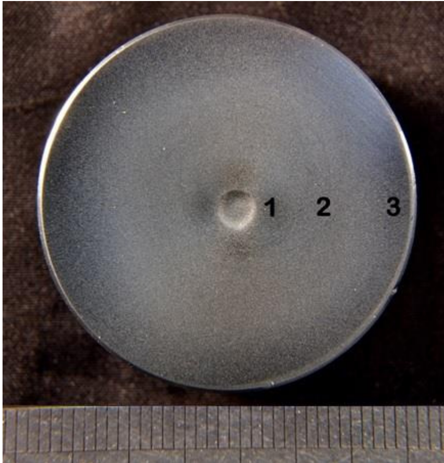
Figure 11. Surface of UNS 31600 after solid/liquid impingement with the three different regions beyond the wear scar.
