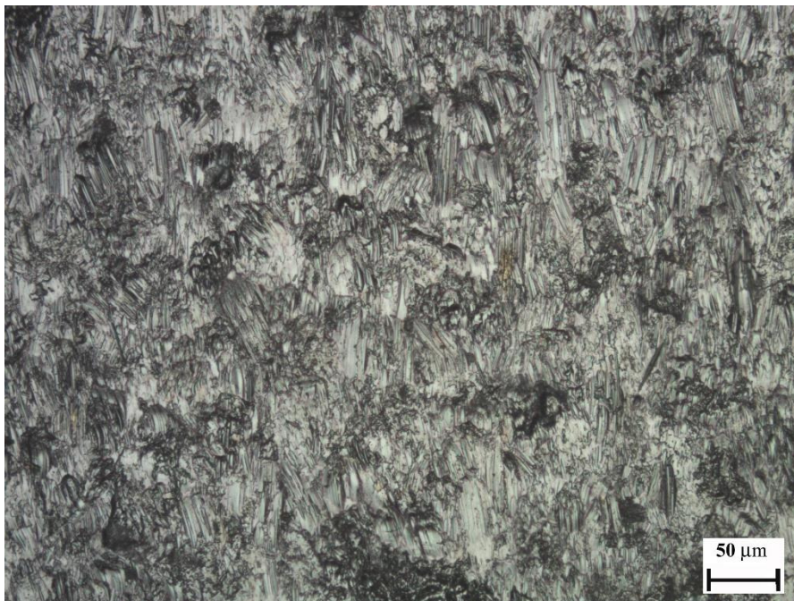
Figure 12. Turbulent area (1) of the UNS S31600 with abrasion marks after solid/liquid impingement.
