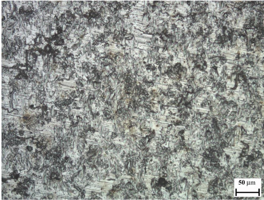
Figure 15. Outermost area (3) of the UNS G1040 after solid/liquid impingement
