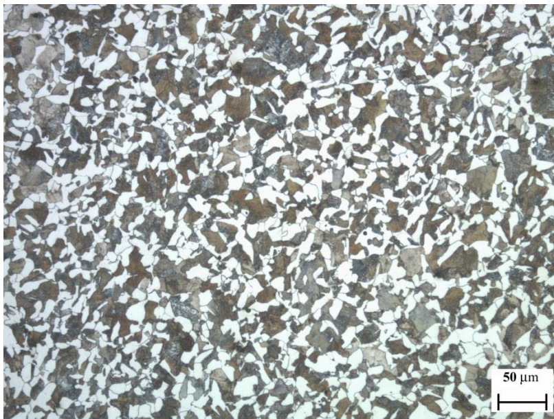
Figure 5. Typical ferrite/pearlite structure of medium carbon steel in UNS G10400
