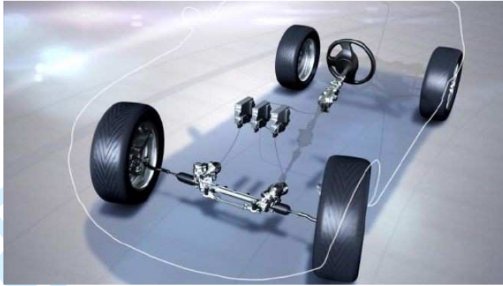
Figure 4. Steer-by-wire system with redundant electronic control units, a backup clutch system that would connect the steering wheel to the tires mechanically if a power failure occur (Picture: Nissan Motors).
