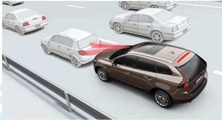
Figure 13. Automatic braking to avoid low-speed frontal crashes (Volvo City Safety system – from Distner et. al [59]).
