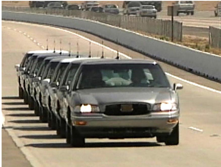
36 37 38 39 40 41 42 43 44 45 46 47 48 49 Figure 6. Live proof-of-concept demonstration of a prototype automated highway system, with self-driving cars operating over a four-day trial period on dedicated lanes of Interstate 15 in San Diego, California 1997 (Photo: California PATH Program).
