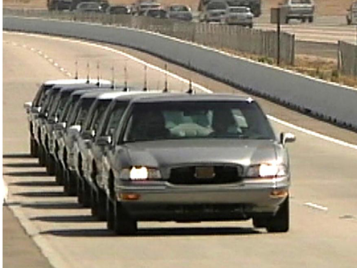
Figure 6. Live proof-of-concept demonstration of a prototype automated highway system, with self-driving cars operating over a four-day trial period on dedicated lanes of Interstate 15 in San Diego, California 1997 (Photo: California PATH Program).
