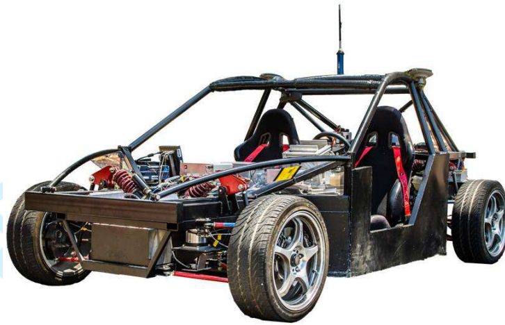
Figure 19. Steer-by-wire test vehicle X1 from Dynamic Design Lab, Stanford. (from Funke [103]).
