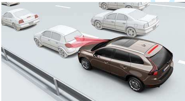
Figure 13. Automatic braking to avoid low-speed frontal crashes (Volvo City Safety system – from Distner et. al [60]).
