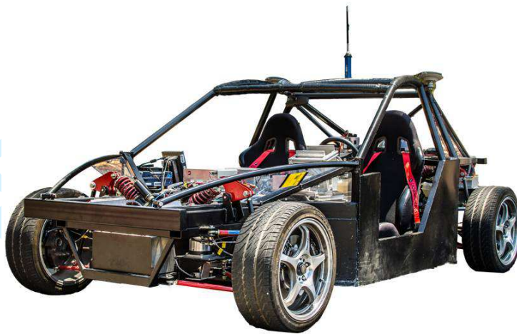
23 Figure 19. Steer-by-wire test vehicle X1 from Dynamic Design Lab, Stanford (from Funke [105]). 24 25
