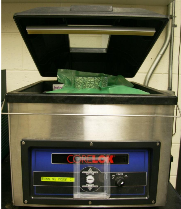
Figure 6-27 CoreLok machine for G_{mb} tests.
