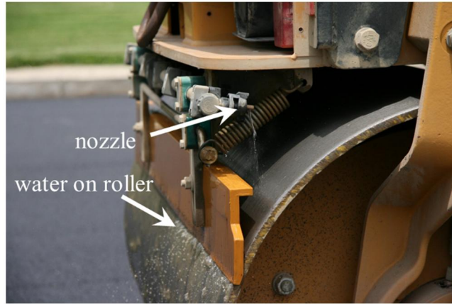
Figure 1-1 Compactor sprays water on the roller during compaction.
