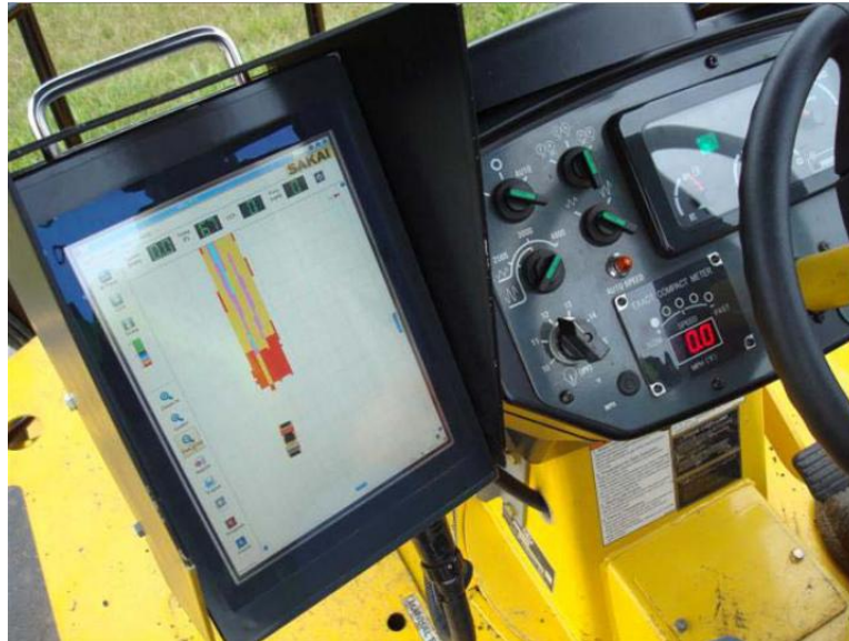
Figure 2-4 Compaction information system on a Sakai asphalt IC roller (36).
