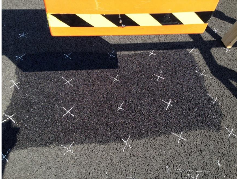
Figure 6-9 Moisturized area under the GPR antenna after spraying 150 mL water.
