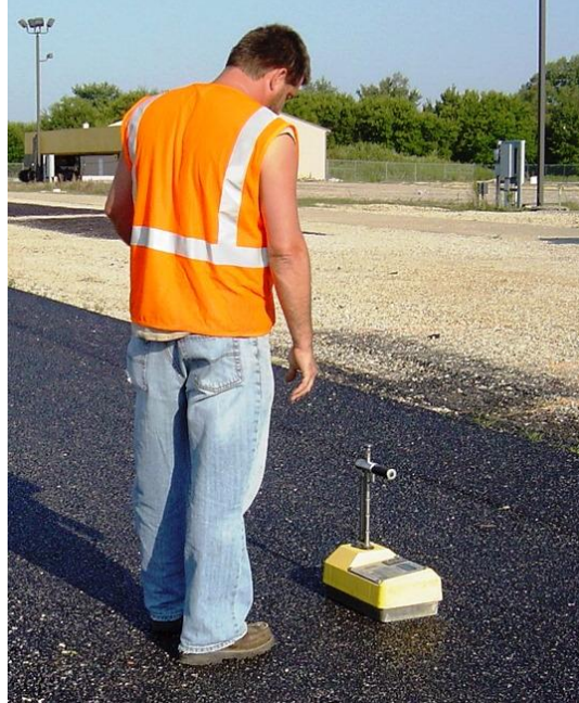
Figure 2-2 Use of nuclear density gauge on measuring asphalt pavement density.
