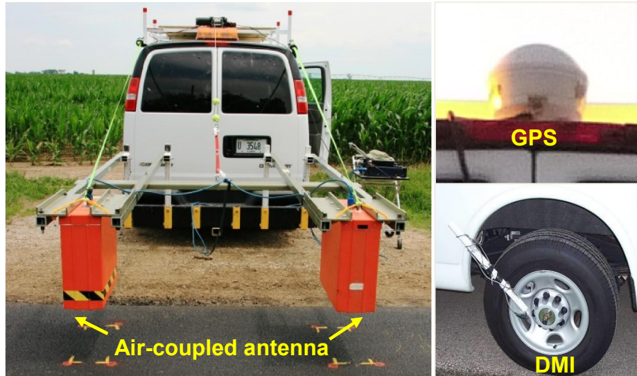
Figure 2-7 Components of a vehicle-mounted air-coupled GPR system.
