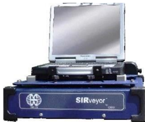
Figure 2-6 Control unit of a GPR system.
