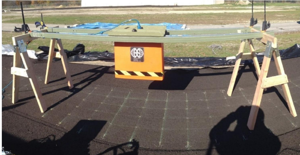
Figure 3-12 Setup of GPR antenna during data collection on test site B.
