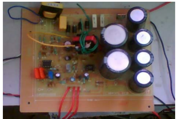
Fig. 13 Experimental setup of flyback buck-boost converter
