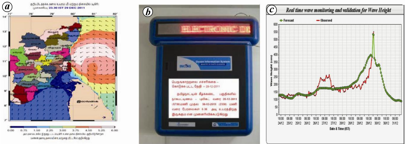
Figure 3. a , The forecast image issued during tropical cyclone Thane for Puducherry and Tamil Nadu. b , High wave alerts displayed through electronic display boards. c , On-line and real-time validation posted at the INCOIS website.
